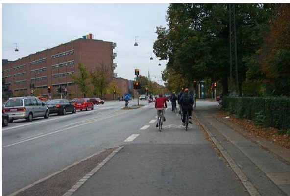
Figure 8. Cycle track dropping to bike lane before an intersection
