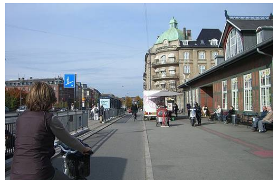
Figure 21. Cycle track passing between bus stop and sidewalk
