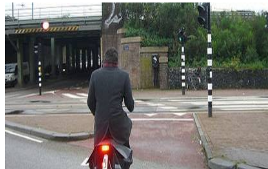
Figure 20. Cycle track crossing streetcar tracks, with pavement yield markings
