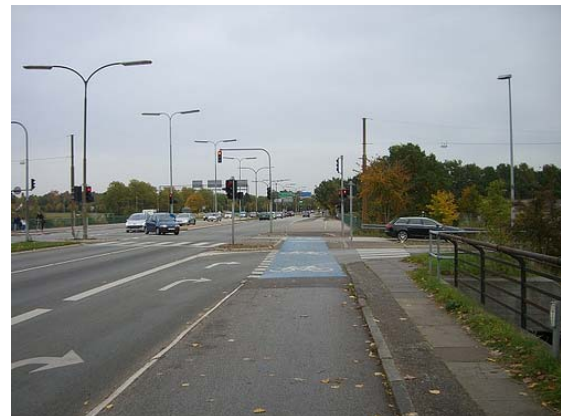
Figure 4. Cycle track is unbroken at driveway crossing
