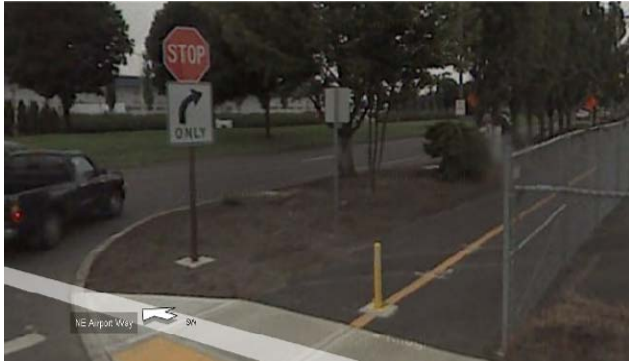
Figure 24. Two-way cycle track on Airport Way in Portland, OR (Source: Google Street View)
